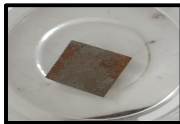
Figure 18. Iron Plate Coated with SiMn Layer 0.6 gr : 0.4 gr After Immersion
