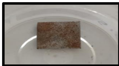
Figure 12. Iron Plate Without Plating After Immersion
