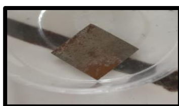
Figure 14. Iron Plate Coated with SiMn Layer 0.4 gr : 0.6 gr After Immersion
