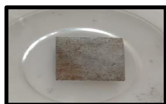
Figure 16. Iron Plate Coated SiMn Layer 0.5 gr : 0.5 gr After Immersion
