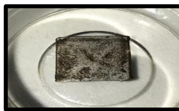
Figure 17. Iron Plate Coated with SiMn Layer 0.6 gr : 0.4 gr Before Immersion
