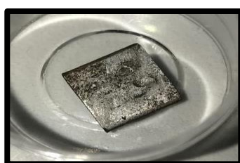
Figure 15. Iron Plate Coated SiMn Layer 0.5 gr : 0.5 gr before immersion
