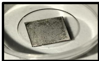
Figure 13. Iron Plate Coated with SiMn Layer 0.4 gr : 0.6 gr Before Immersion
