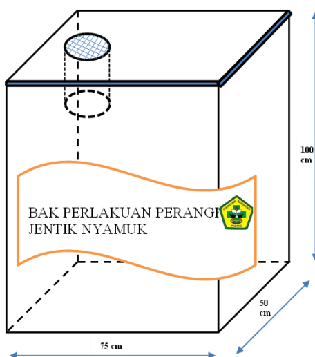
Fig.1 Sketch of the Engineered Basin in the Treatment for Potential Breeding Sites Mosquitoes Aedes aegypti
